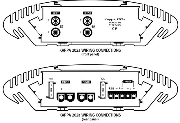
Figure 7. Wiring connections for the Kappa 202a amplifier.
